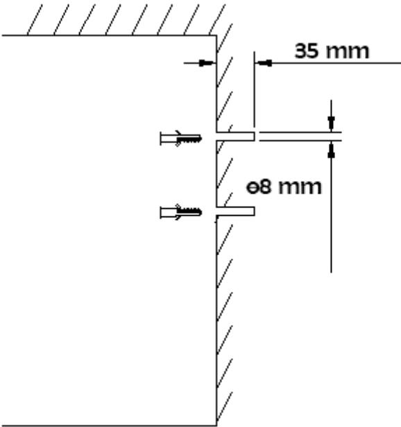
Step 3: Attach the wall bracket to the wall using the screws.
