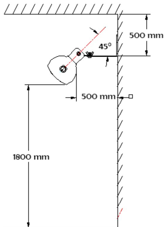
Make sure the mounting wall isn't made of combustible materials (e.g. wood). Check exterior walls for communication and electrical cables and pipelines. Should any service lines be present in the immediate vicinity, do not install the heater there and find an alternative location.
